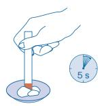
Bring the activated stick into direct contact with the substance to be tested for at least 5 seconds.
