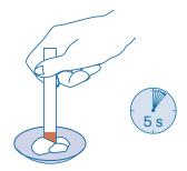
Bring the activated stick into direct contact with the substance to be tested for at least 5 seconds.
