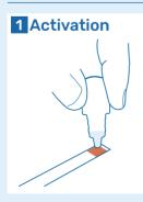
Moisten the pad by briefly holding the Activator vial vertically against the pad of the stick. An automatic outflow takes place. Do not press the vial. Only use a small amount of the Activator liquid. The red dye will be activated and remains active for about 15 minutes.
