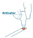
Moisten the pad by briefly holding the Activator bottle against the pad. The Activator will flow out automatically. The red dye is activated and remains active for about 15 minutes.
